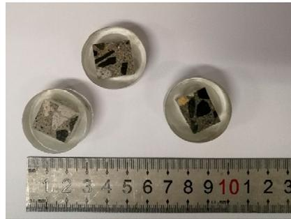
**Figure 4.** The samples for nanoindentation test.
