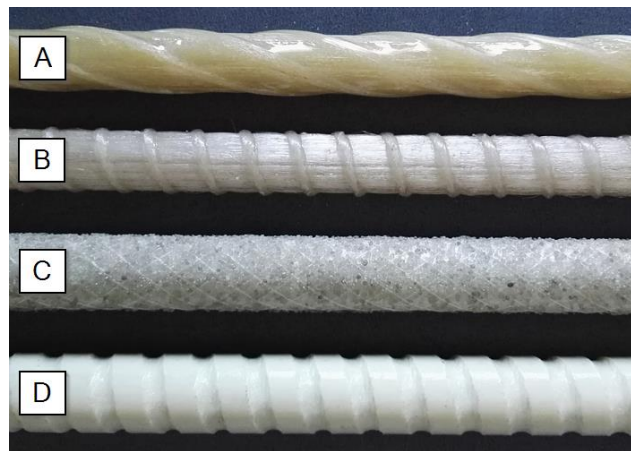
Figure 1. Types of tested GFRP bars. (A) AlbaKompozit; (B) ComRebars; (C) Pultrall; (D) Schoeck.
