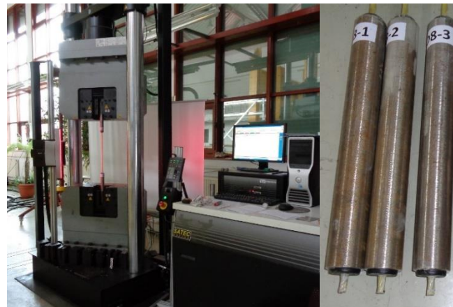
Figure 2. Exemplary GFRP bar gripped in the testing machine ( left ) and anchorages of bars ( right ).
