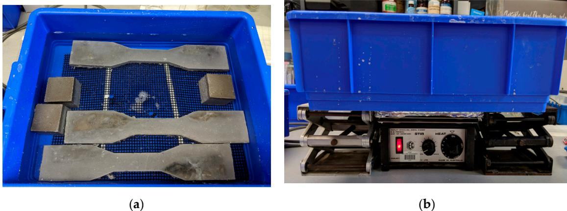
Figure 5. (a,b). Sulfuric acid bath with magnetic stirrer.
