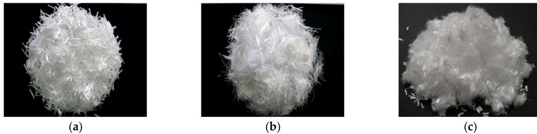
Figure 3. Fiber type: (a) Polyethylene (PE); (b) polypropylene (PP); (c) nylon (NY).
