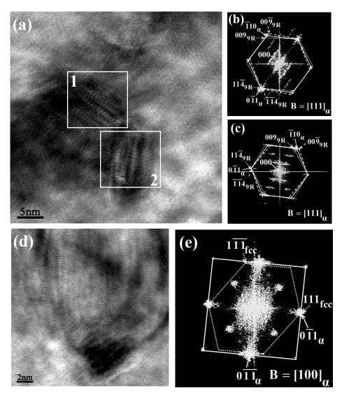
**Figure 4.** HRTEM images and their fast Fourier transform (FFT) patterns of Cu precipitates: (**a**) twinned 9R Cu image after aging for 1 h; (**b**) the FFT pattern of the square region 1 marked in (**a**); (**c**) the FFT pattern of the square region 2 marked in (**a**); (**d**) stable fcc Cu image after aging for 3 h; and (**e**) the FFT pattern of (**d**).
