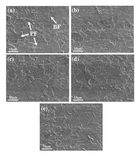
**Figure 2.** SEM images of the tested steel samples: (**a**) after water cooling; and after aging at 500 °C for (**b**) 0.5 h; (**c**) 1 h; (**d**) 1.5 h; and (**e**) 3 h.
