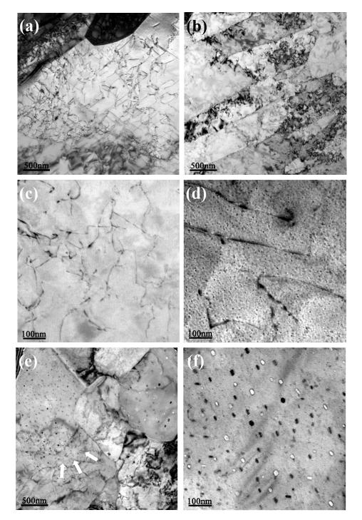
**Figure 3.** Bright-field TEM images of the tested steel samples for: (**a**) high density dislocations after water cooling; (**b**) bainitic ferrite laths after water cooling; (**c**) low density dislocations after aging for 0.5 h; (**d**) fine Cu precipitates after aging for 1 h; (**e**) recovery of the matrix showing the annihilation of dislocations and growth of Cu precipitates after aging for 3 h; and (**f**) coarsened Cu precipitates after aging for 3 h.
