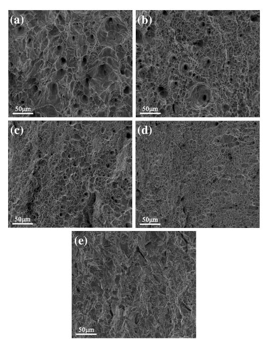
**Figure 8.** SEM micrographs showing the impact fracture surfaces at -80 °C after: (**a**) water cooling; and aging for (**b**) 0.5 h; (**c**) 1 h; (**d**) 1.5 h; and (**e**) 3 h.
