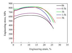
Figure 6. Tensile stress-strain curves of the steel samples subjected to different processing methods.
