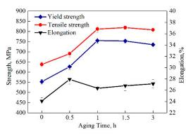
Figure 5. Variation of yield strength, tensile strength and elongation as a function of aging time.
