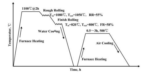
Figure 1. Schematic of the processing methods used in this study.
