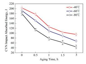
Figure 7. The Charpy V-notch (CVN) impact absorbed energies of the tested steel samples.
