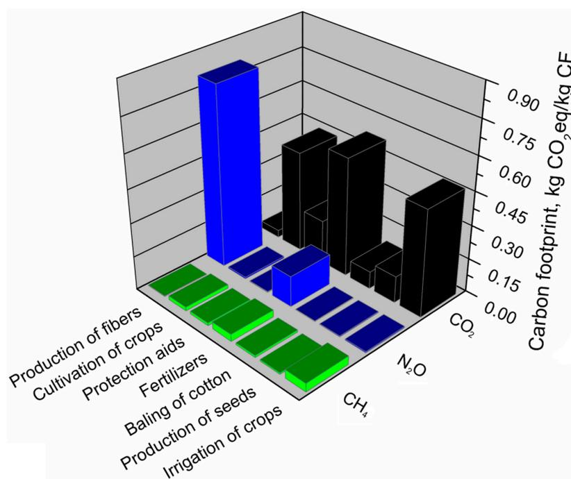
**Figure 12.** Shares of individual GHGs emissions in the main components of the cotton fibers production system.
