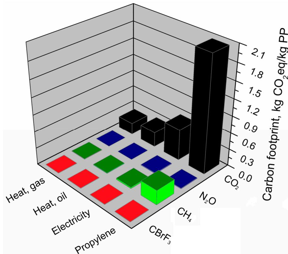
**Figure 11.** Shares of individual GHG emissions in the main components of the polypropylene production system.
