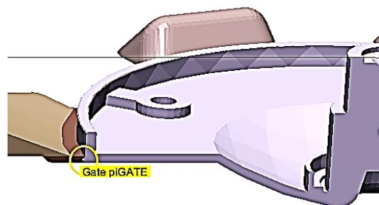
**Figure 7.** The location of the melt temperature evaluation in the gate.
