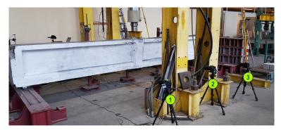
**Figure 9.** Test stand prepared for monitoring post-tensioned, precast crane runway beam during the three-point bending test using the CivEng Vision system.
