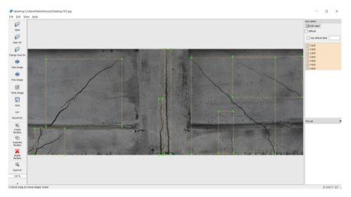
Figure 6. Example of annotation of an image of concrete element containing several cracks.
