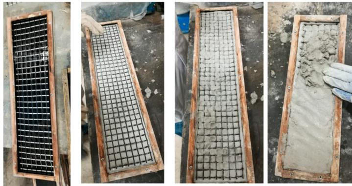
Figure 3. Production stages of composites produced using the M60 matrix.
