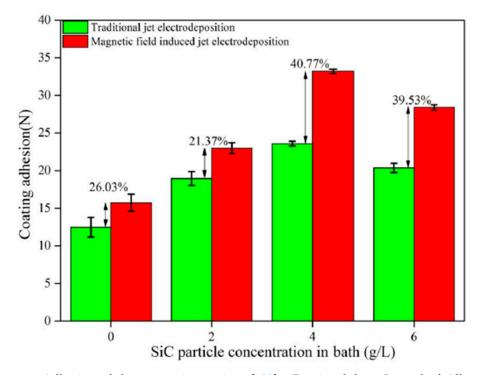
**Figure 12.** Adhesion of the composite coatings [120]. Reprinted from Journal of Alloys and Compounds, 791, Wei Jiang, Lida Shen, Mingyang Xu, Zhanwen Wang, Zongjun Tian, Mechanical properties and corrosion resistance of Ni–Co–SiC composite coatings by magnetic field-induced jet electrodeposition/Pages No. 847–855, Copyright (2020), with permission from Elsevier.
