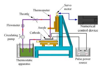
Figure 1. Schematic image of pulse jet electrodeposition.
