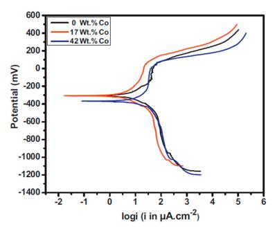
**Figure 13.** The potentiodynamic polarization curves of the Ni–Co alloy coating as a function of the cobalt content [126]. Reprinted from Applied Surface Science, 307, Babak Bakhit, Alireza Akbari, Farzad Nasirpouri, Mir Ghasem Hosseini, Corrosion resistance of Ni–Co alloy and Ni–Co/SiC nanocomposite coatings electrodeposited by sediment codeposition technique/Pages No. 351–359, Copyright (2020), with permission from Elsevier.
