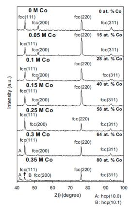
**Figure 7.** X-ray diffraction (XRD) patterns of Ni–Co films deposited from the electrolytes containing different Co concentrations [68]. Reprinted from Applied Surface Science, 258, Ali Karpuz, Hakan Kockar, Mursel Alper, Oznur Karaagac, Murside Haciismailoglu, Electrodeposited Ni–Co films from electrolytes with different Co contents/Pages No. 4005–4010, Copyright (2020), with permission from Elsevier.
