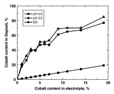
**Figure 6.** Alloy composition as a function of Co<sup>2+</sup> concentration in the electrolyte [16]. Reprinted from Surface and Coatings Technology, 201, Meenu Srivastava, V. Ezhil Selvi, V.K. William Grips, K.S. Rajam, Corrosion resistance and microstructure of electrodeposited nickel-cobalt alloy coatings/Pages No. 3051–3060, Copyright (2020), with permission from Elsevier.
