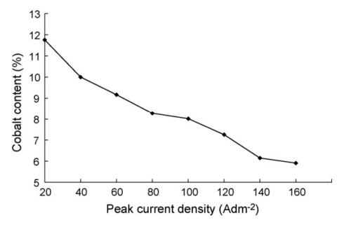
**Figure 3.** Cobalt content in Ni–Co alloy coatings with varying peak current density [34]. Reprinted from Applied Surface Science, 254, Yundong Li, Hui Jiang, Weihua Huang, Hui Tian, Effects of peak current density on the mechanical properties of nanocrystalline Ni–Co alloys produced by pulse electrodeposition/Pages No. 6865–6869, Copyright (2020), with permission from Elsevier.
