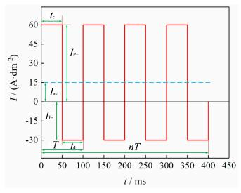
**Figure 2.** Schematic diagram of pulse waveform when  $I_{av} = 15 \text{ A} \cdot \text{dm}^2$ ,  $\lambda = 0.5$ , x = 0.5, and f = 10 Hz.
