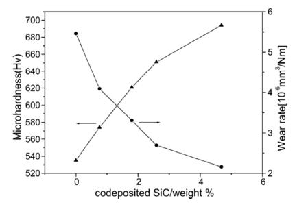
**Figure 10.** Microhardness and wear rate of the nanocomposite coating vs. weight percentage of co-deposited SiC particulates in the nanocomposite coating [60]. Reprinted from Applied Surface Science, 252, Lei Shi, Chufeng Sun, Ping Gao, Feng Zhou, Weimin Liu, Mechanical properties and wear and corrosion resistance of electrodeposited Ni–Co/SiC nanocomposite coating/Pages No. 3591–3599, Copyright (2020), with permission from Elsevier.
