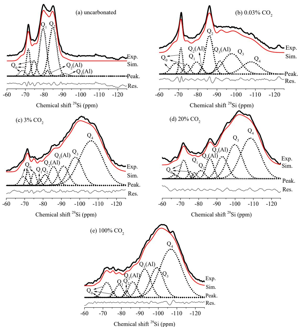
**Figure 4.** NMR spectra of slag blended cement pastes with and without carbonation: (a) uncarbonated; (b) 0.03% CO<sub>2</sub>; (c) 3% CO<sub>2</sub>; (d) 20% CO<sub>2</sub>; (e) 100% CO<sub>2</sub>.
