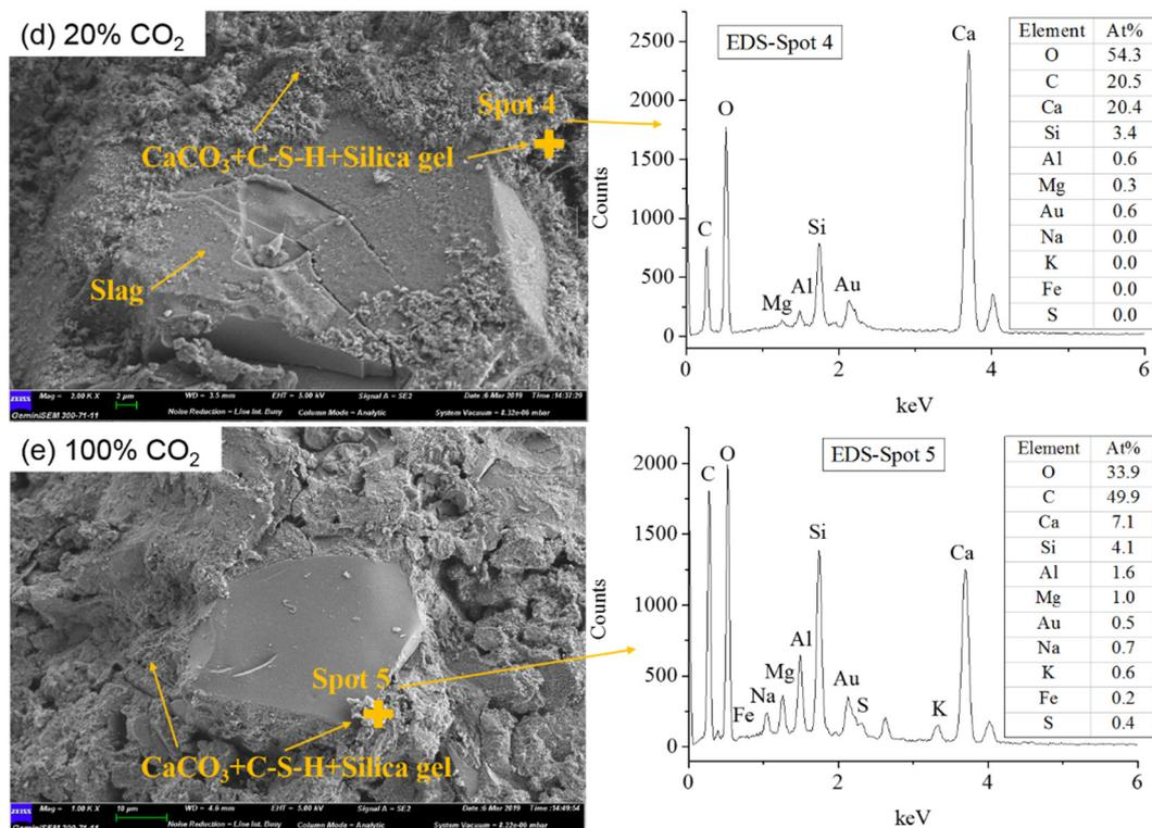
**Figure 6.** SEM images of slag blended cement pastes before and after carbonation with different concentrations: (a) uncarbonated, (b) 0.03% CO<sub>2</sub>, (c) 3% CO<sub>2</sub>, (d) 20% CO<sub>2</sub>, (e) 100% CO<sub>2</sub>.
