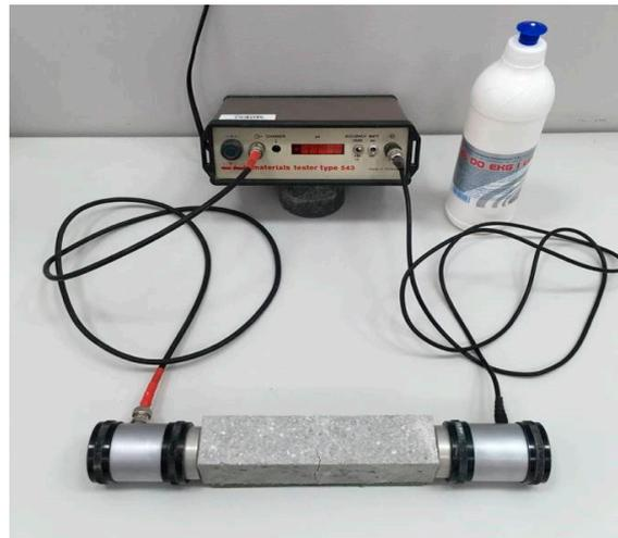
**Figure 4.** Test stand for testing the ultrasonic pulse velocity by direct transmission in rectangular mortar samples.
