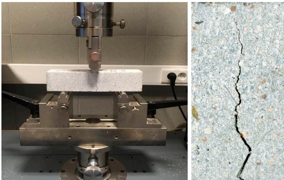
**Figure 2.** Sample immediately after the induction of the defect by three-point bending, and a typical image of the single crack with variable width (side wall of the sample, parallel to the force direction).
