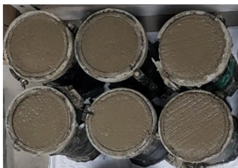
Figure 3. Specimen for chloride ion migration coefficient.
