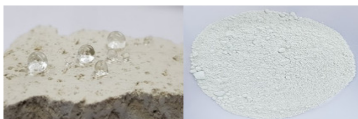
Figure 1. Water-repellent impregnated natural zeolite.
