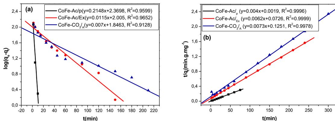
**Figure S6.** (a) Pseudo-first-order and (b) pseudo-second-order kinetics for adsorption of direct red 2 on CoFeAc/p, CoFe-Ac/Ex, and CoFe-CO<sub>3</sub>/A LDHs.
