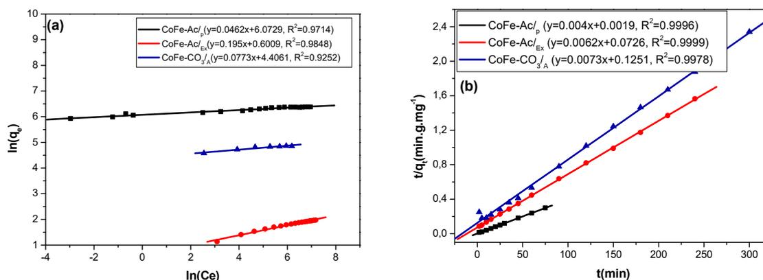
**Figure S7.** (a) Freundlich and (b) Langmuir isotherms for adsorption of direct red 2 on CoFe-Ac/p, CoFe-Ac/Ex, and CoFe-CO<sub>3</sub>/A LDHs.
