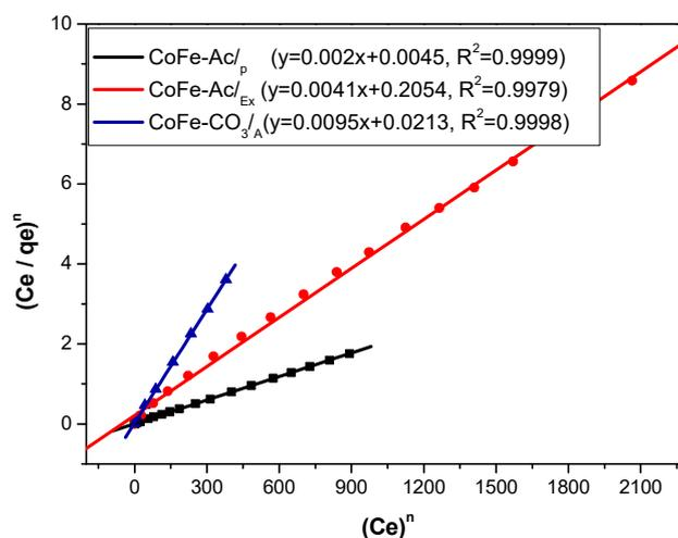
**Figure S8.** Toth isotherm for adsorption of direct red 2 on CoFe-Ac/p, CoFe-Ac/Ex, and CoFe-CO<sub>3</sub>/A LDHs.
