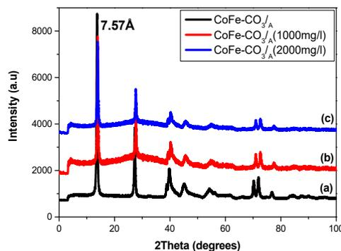
**Figure S10.** X-ray diffractogram before and after adsorption for CoFe-CO<sub>3</sub>/A.
