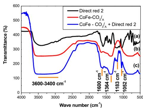
**Figure S9.** FT-IR spectra before and after adsorption for CoFe-CO<sub>3</sub>/A.
