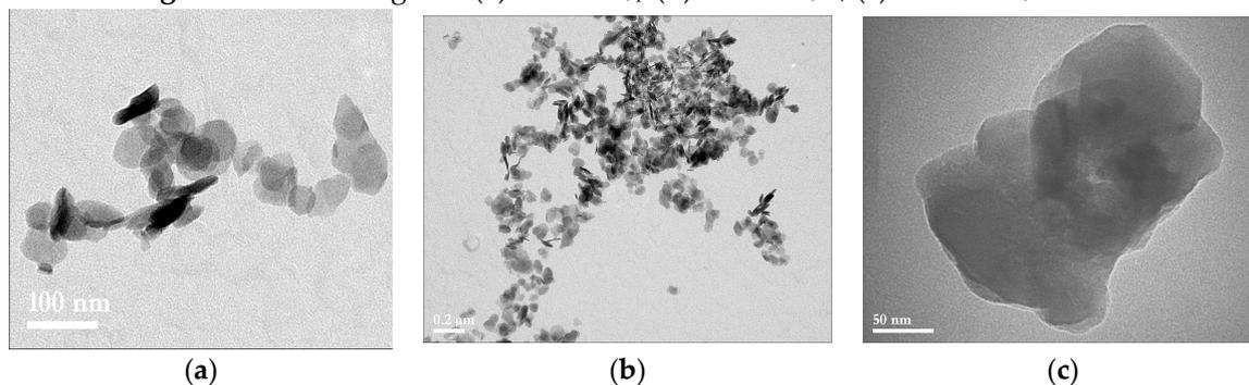
**Figure S2.** TEM images of (a) CoFe-Ac/p, (b) CoFe-Ac/Ex, (c) CoFe-CO<sub>3</sub>/A LDHs.
