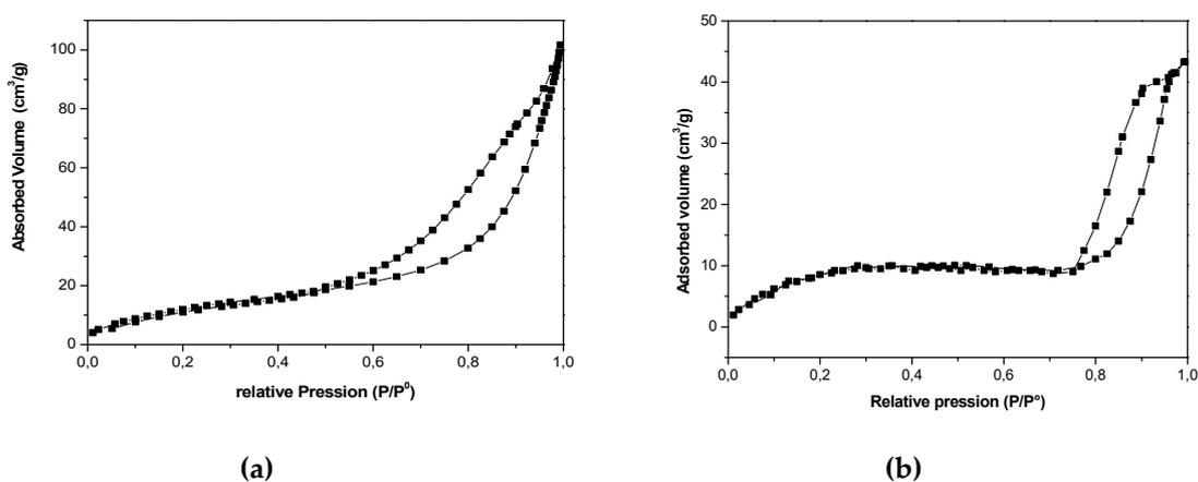
Figure S5. N<sub>2</sub> adsorption–desorption isotherms of (a) CoFe-Ac/p (b) CoFe-Ac/Ex LDHs
