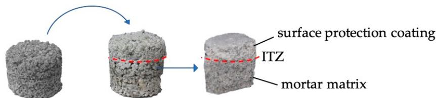
**Figure 1.** Schematic representation of a mortar before and after the application of the surface protection cementitious coatings.
