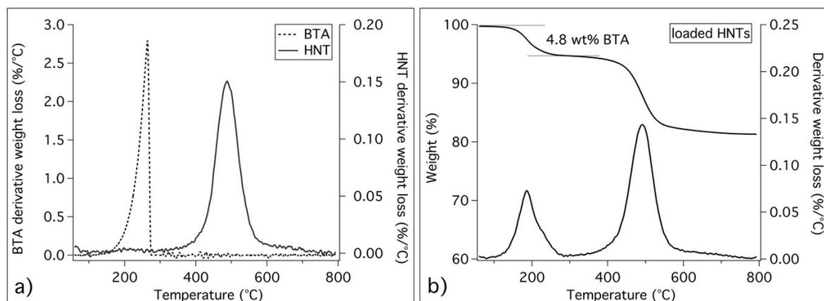
**Figure 2.** Thermogravimetric curves: (a) derivative thermogravimetry (DTG) curves of pristine benzotriazole (BTA) and halloysite nanotubes (HNTs); (b) thermogravimetry (TG)/DTG curves of loaded HNTs, together with the evaluation of BTA weight amount in loaded nanotubes.
