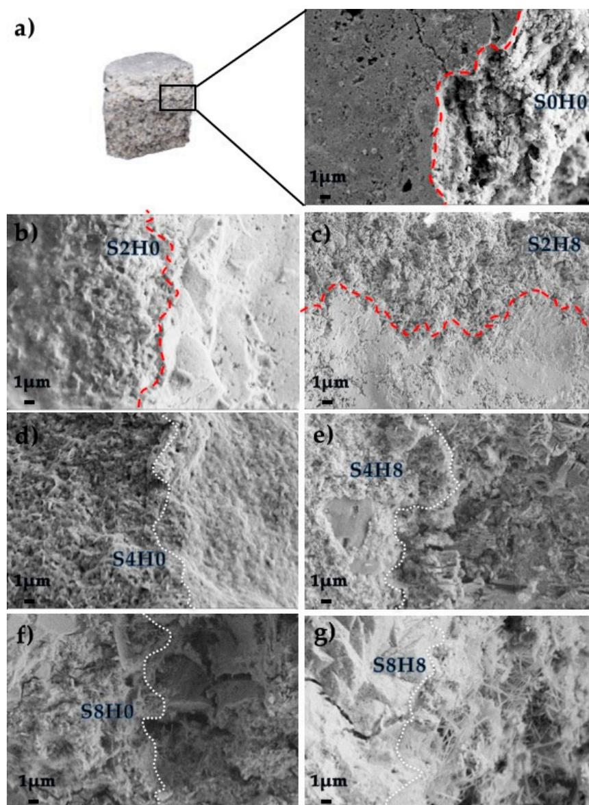
**Figure 5.** SEM images of top coating/bottom matrix interphases: (a) sketch of the interphase and morphology of the ITZ bottom matrix/S0H0 coating; (b) ITZ bottom matrix/S2H0 coating; (c) ITZ bottom matrix/S2H8 coating; (d) ITZ bottom matrix/S4H0 coating; (e) ITZ bottom matrix/S4H8 coating; (f) ITZ bottom matrix/S8H0 coating; (g) ITZ bottom matrix/S8H8 coating.
