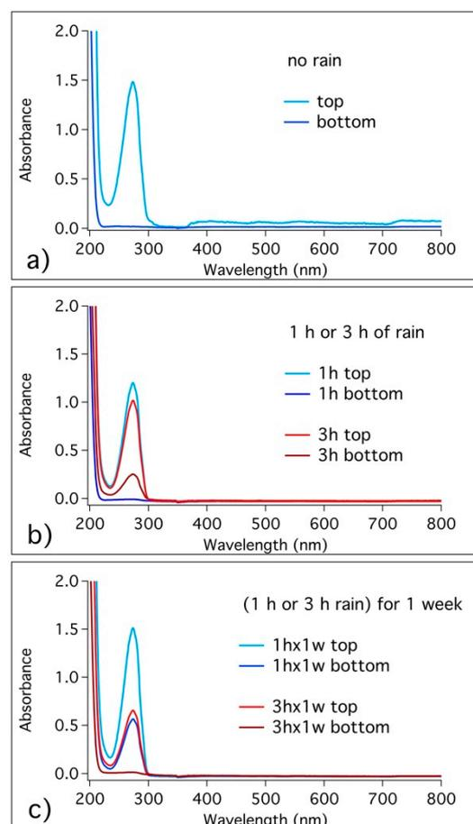
**Figure 9.** UV-vis spectra of the top and bottom piece solutions for surface coated surfaces under different conditions of rain: (a) no rain; (b) 1 h and 3 h of moderate rain; (c) 1 h and 3 h of moderate rain repeated for 1 week.
