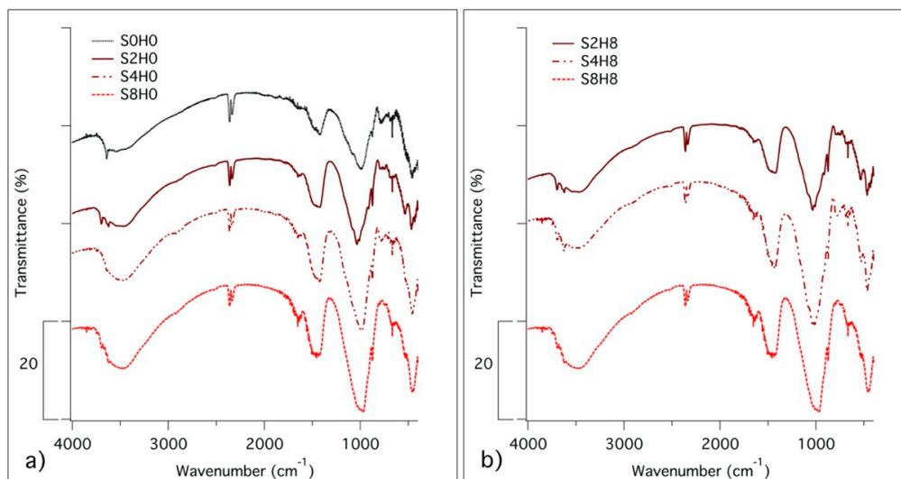
**Figure 4.** FTIR spectra of (a) S0H0, S2H0, S4H0 and S8H0; (b) S2H8, S4H8, S8H8. Samples have been lyophilized and analysed after 28 days of hydration. Spectra have been offset for the sake of clarity.
