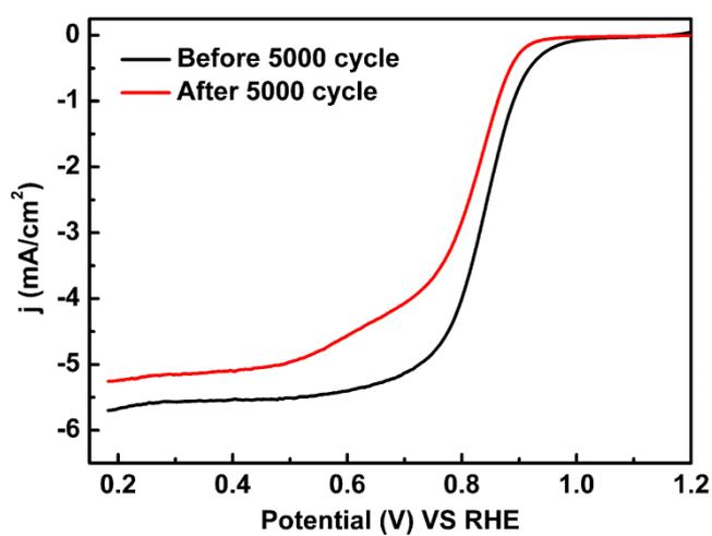
Figure S8. Cycling stability of 20% commercial Pt/C catalysts in 0.1 M KOH solution under 1600 rpm.
