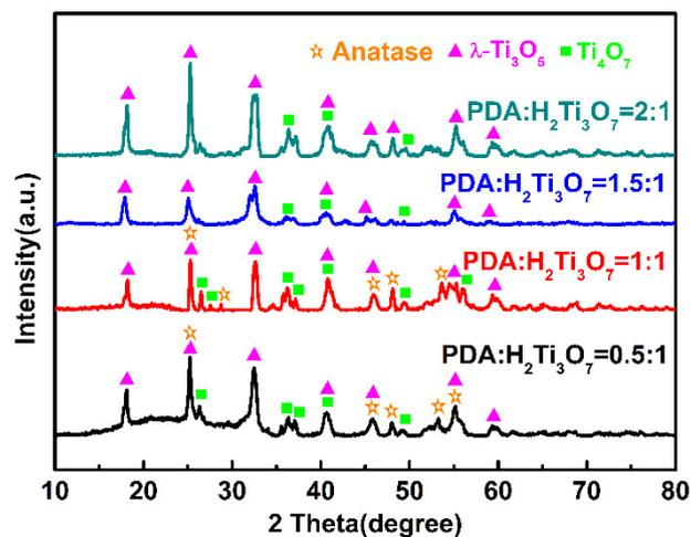
Figure S4. XRD spectra of the  $\text{Ti}_n\text{O}_{2n-1}$  nanofibers with different content of PDA.
