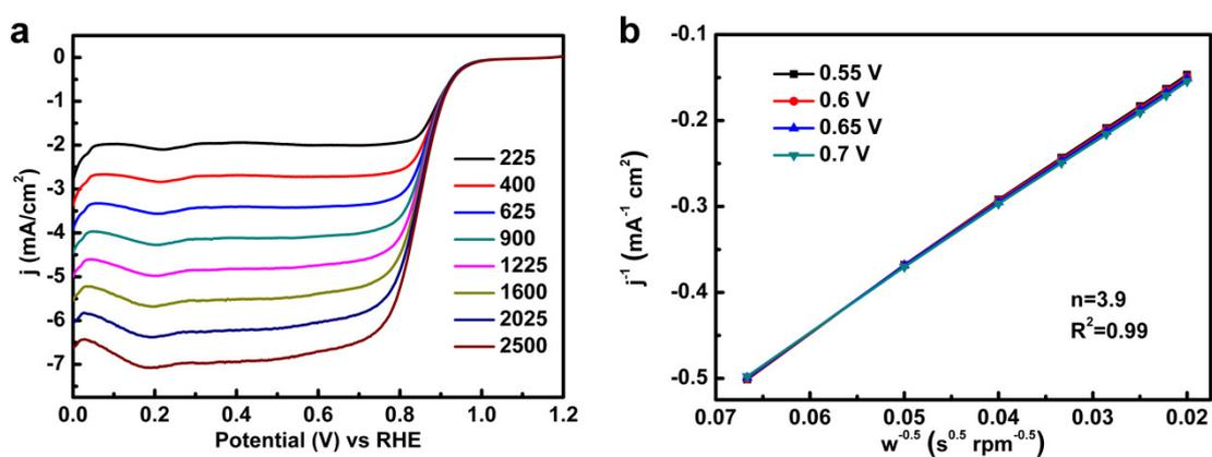
Figure S6. The ORR catalytic performance of 20% commercial Pt/C in 0.1 M KOH solution.
