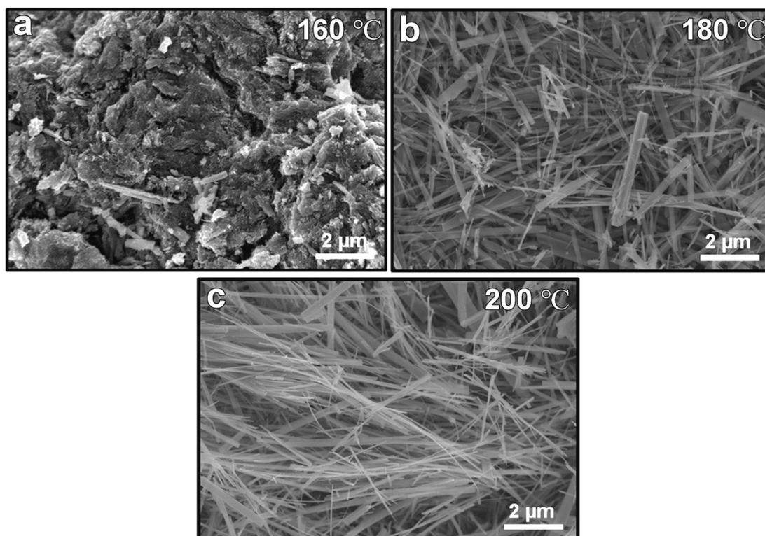
Figure S2. SEM images of the  $H_2Ti_3O_7$  nanofibers under different hydrothermal reaction temperatures.
