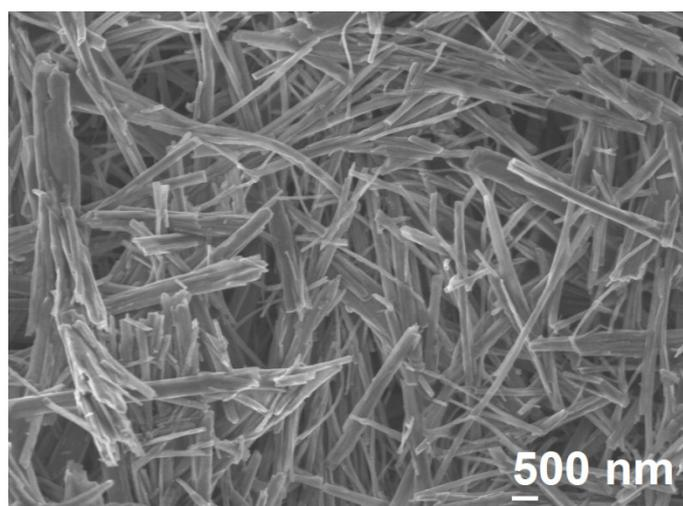
Figure S9. SEM image of T4/T3 nanofibers after the long time working.
