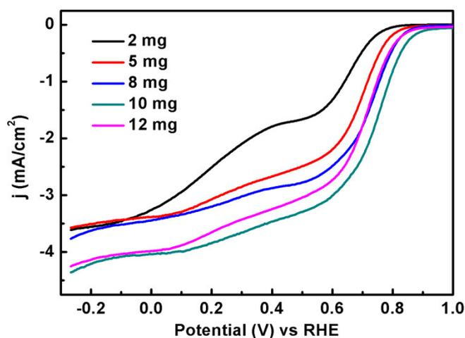
Figure S5. The effect of catalysts loading amount on the ORR performance.
