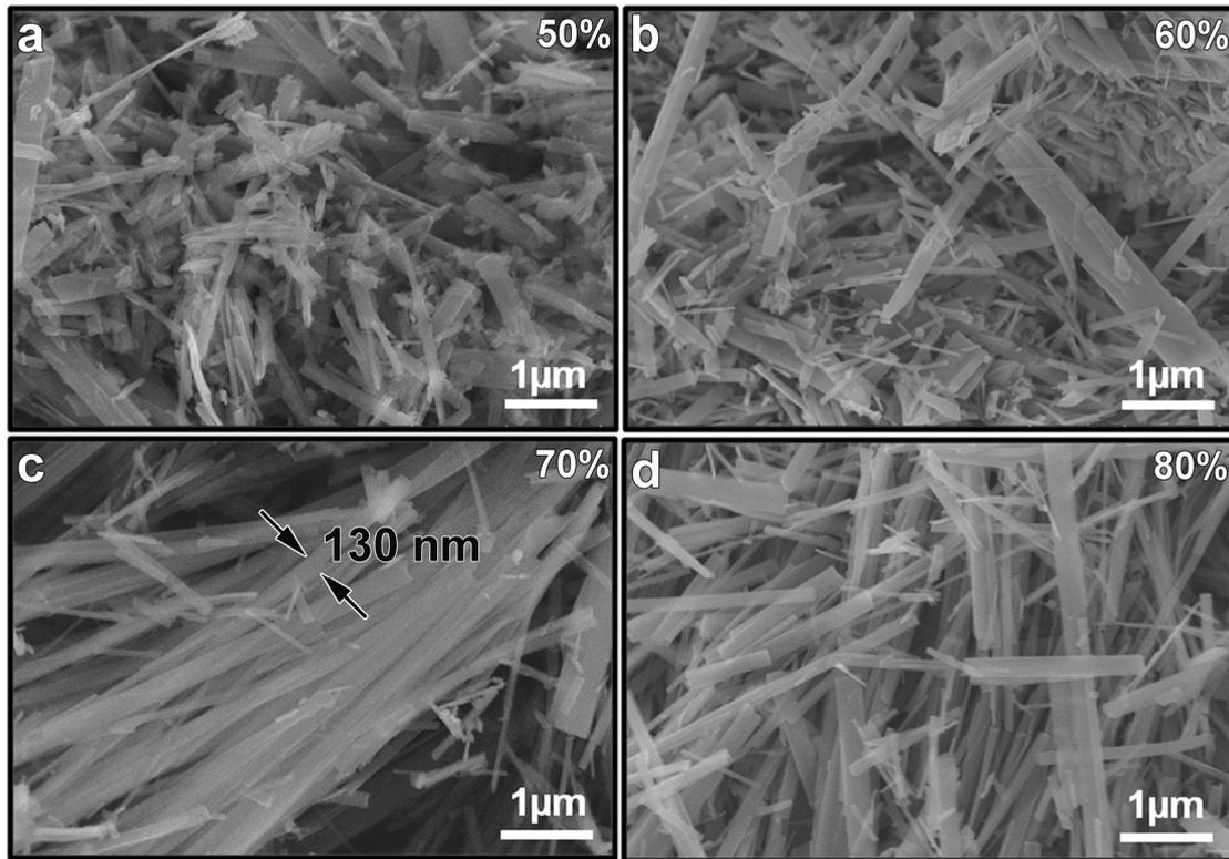
**Figure S1.** SEM images of the obtained  $\text{H}_2\text{Ti}_3\text{O}_7$  nanofibers under different filling amount of the reactor.
