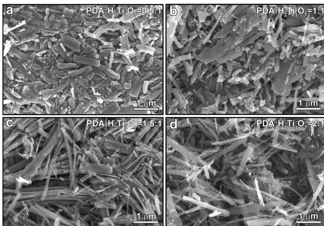
Figure S3. SEM images of the obtained  $Ti_{n-1}O_{2n-1}$  nanofibers with different PDA:  $H_2Ti_3O_7$  weight ratio.
