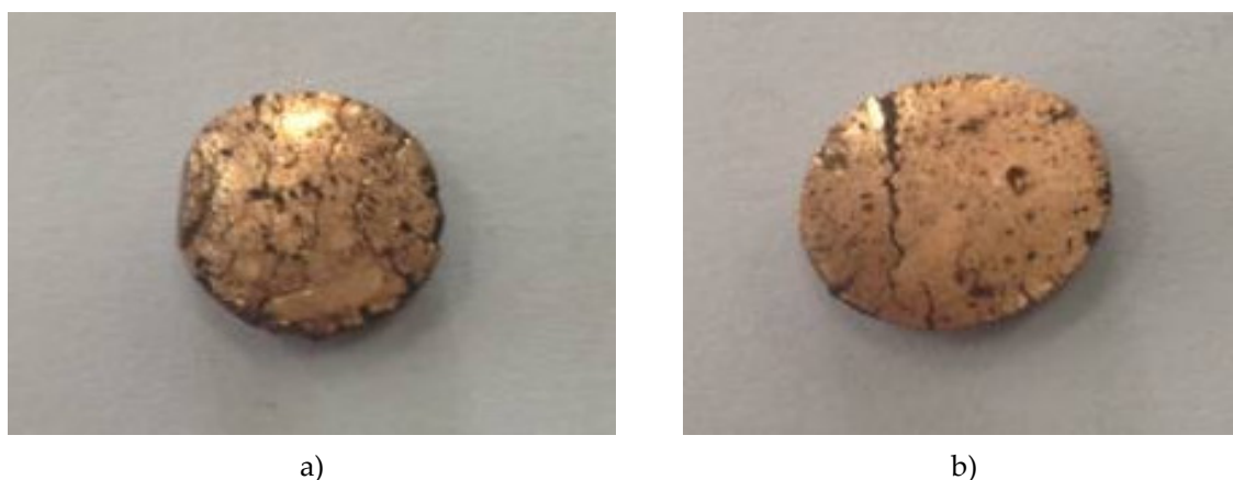
Figure 19. Images of Cu-5%Fe 3 O 4 (a) and Cu-15%Fe 3 O 4 (b) nanocomposites after cold rolling.
