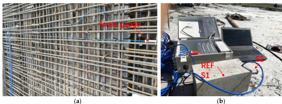
Figure 3. Field arrangement of strain gauge: (a) placement of strain gauge; (b) data acquisition.
