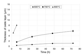
Figure 2. Results of thickness measurements of oxide scales depending on annealing parameters.
