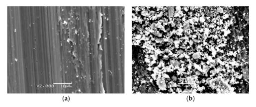
**Figure 12.** Microscopic photographs of the friction path formed on titanium after tests with Al<sub>2</sub>O<sub>3</sub> balls (corrugation wear: (a) light grey zone, (b) dark grey zone).
