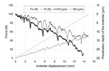
**Figure 6.** Scratch behavior of titanium Grade 2 in the non-oxidized condition ( $F_n$ —indenter load,  $F_t$ —resistance to indenter penetration,  $P_d$ —depth of indenter penetration under load,  $R_d$ —depth of indenter penetration after unloading).
