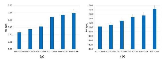
Figure 15. Surface roughness of titanium after annealing at 600, 700 and 800 °C (parameters (a) R<sub>a</sub>, (b) R<sub>z</sub>).
