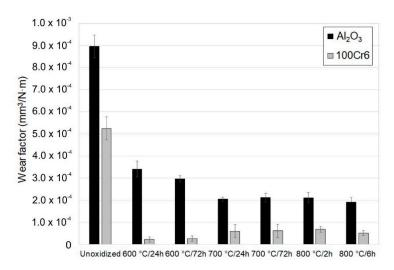
**Figure 8.** Wear factor of titanium before and after annealing in a ceramic (Al<sub>2</sub>O<sub>3</sub>) and metallic (bearing steel 100Cr6) tribological couple.
