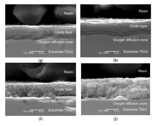
**Figure 1.** Cross-sectional area of titanium with an oxide scale obtained at a temperature of: 600 °C for (a) 6 h, (b) 24 h, (c) 48 h and (d) 72 h; (e) 700 °C for 6 h, (f) 24 h, (g) 48 h and (h) 72 h; (i) 800 °C for 2 h and (j) 6 h.
