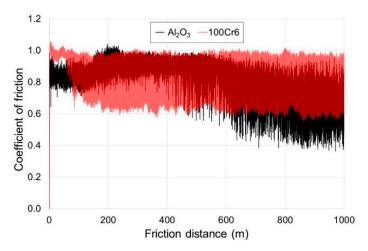
**Figure 11.** Diagram of the friction coefficient for titanium after annealing at 700  $^{\circ}$ C (72 h), recorded during friction with Al<sub>2</sub>O<sub>3</sub> and 100Cr6 balls.
