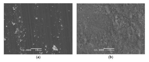
**Figure 14.** Microscopic photographs of the friction path formed on titanium after annealing at 700 °C for 72 h, after tests with (a)  $Al_2O_3$  and (b) 100Cr6 balls.
