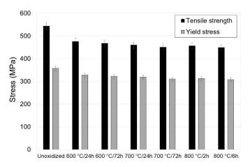
Figure 3. Tensile properties of titanium after annealing.
