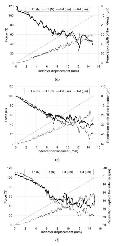
**Figure 7.** Scratch behavior of titanium after annealing at: (a) 600 °C for 24 h, (b) 600 °C for 72 h, (c) 700 °C for 24 h, (d) 700 °C for 72 h, (e) 800 °C for 2 h, (f) 800 °C for 6 h (F<sub>n</sub>—indenter load, F<sub>t</sub>—resistance to indenter penetration, P<sub>d</sub>—depth of indenter penetration under load, R<sub>d</sub>—depth of indenter penetration after unloading).
