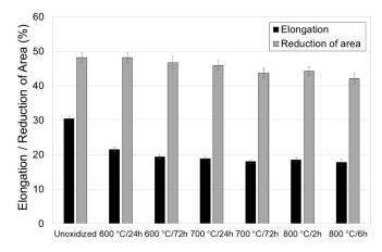
Figure 4. Measurement results of plastic parameters (elongation and reduction in area) for titanium Grade 2.
