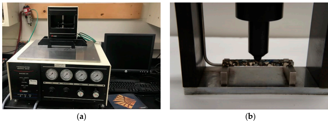
Figure 3. Testing setup of bending beam rheometer (BBR) mixture creep test: (a) BBR testing device, (b) mixture beam sample.
