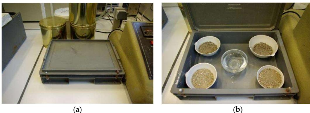
**Figure 1.** Experimental device for water capture measurement from atmospheric air water: (a) closed box in the laboratory with temperature and humidity set at  $20 \pm 3$  °C and  $60 \pm 10\%$ ; and (b) the closed box containing the dried samples and water.
