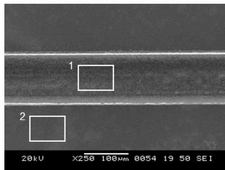
**Figure 11.** Analysis was conducted of the square areas outlined in white. Square 1 indicates the bottom surface of a channel and square 2 indicates the glass surface.
