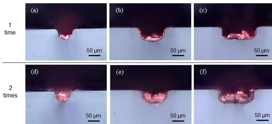
**Figure 9.** Optical images of embedded copper wires from a section view with a single laser scan and widths of (a) 50  $\mu\text{m}$ , (b) 100  $\mu\text{m}$ , and (c) 150  $\mu\text{m}$  and with multiple laser scans and widths of (d) 50  $\mu\text{m}$ , (e) 100  $\mu\text{m}$ , and (f) 150  $\mu\text{m}$ .
