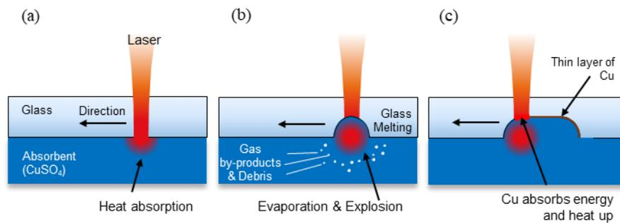
**Figure 1.** Brief mechanism of the LIBWE process: (a) An irradiated laser beam is absorbed by the absorbents. (b) Glass is removed by the heated absorbents. (c) Glass is continuously removed by the heated metal layer and absorbents.
