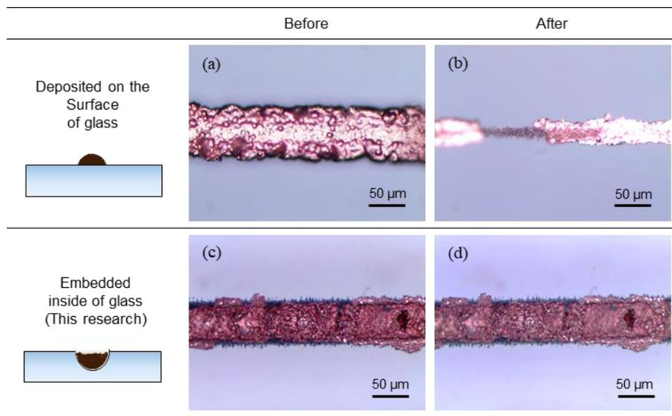
**Figure 10.** Durability test for deposited copper on the surface of the glass (a) before and (b) after the ultrasonic vibration test and inside channels; (c) before; and (d) after the ultrasonic vibration test.
