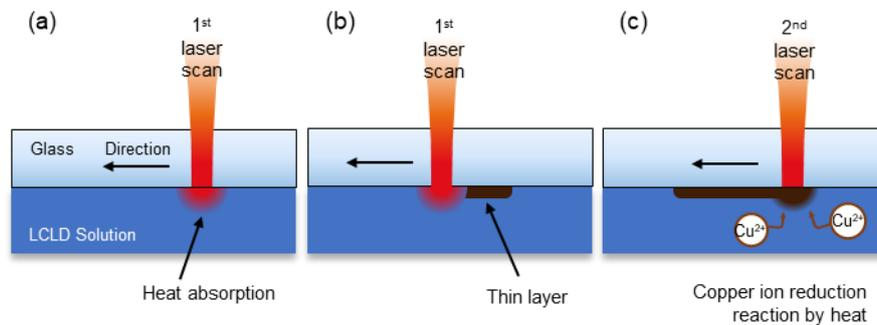
**Figure 2.** Brief mechanism of the LCLD process. (a) The laser beam is absorbed by the solution. (b) The copper ion reduction reaction occurs, and a thin layer of copper attaches to the surface of the glass. (c) Copper grows from the solution.
