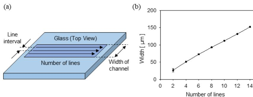
**Figure 6.** Controlling the width of the channels by the number of lines under LIBWE. (a) Definition of the number of lines and the line interval. (b) Fabricated channel widths according to the number of lines.
