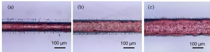
**Figure 8.** Optical images of embedded copper wires from the top view. Widths of (a) 50  $\mu\text{m}$ , (b) 100  $\mu\text{m}$ , and (c) 150  $\mu\text{m}$ .
