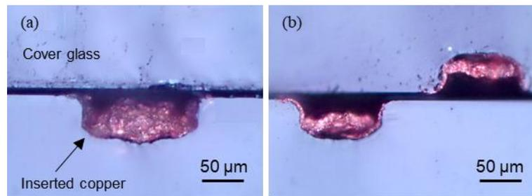
**Figure 13.** Cross section images of (a) a fully filled 150  $\mu\text{m}$  wide channel sealed with cover glass; and (b) two layers of half-filled 100  $\mu\text{m}$  wide channels stacked without supports.
