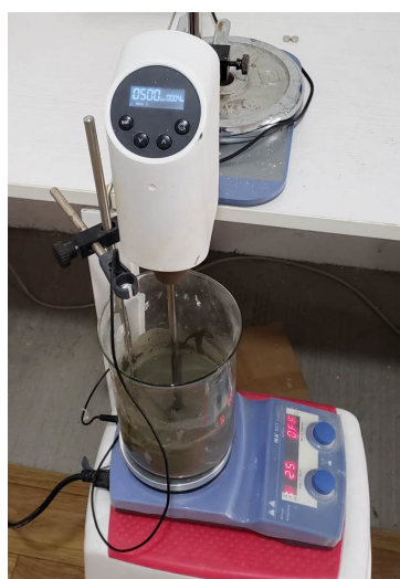
Figure 3. Mixing and temperature control of grouts.
