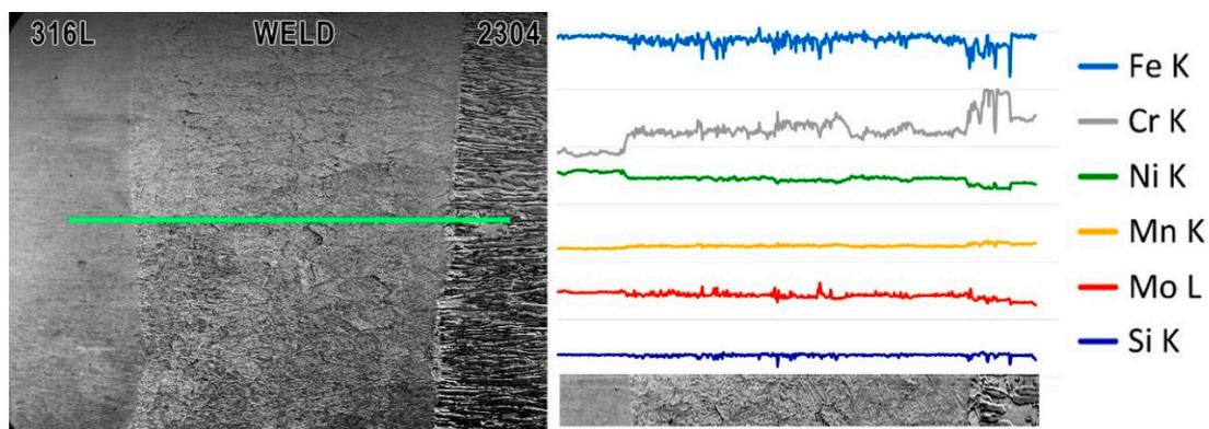
**Figure 9.** Results of EDS linear analysis through the welded joint from 316L austenitic stainless steel (beginning of the line) to 2304 duplex stainless steel (end of the line). The analysis was carried out along the line indicated in the SEM image on the left.
