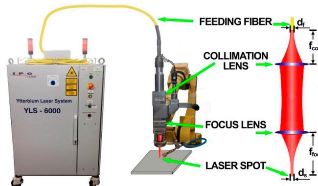
**Figure 1.** Experimental set-up for fiber laser welding [56].
