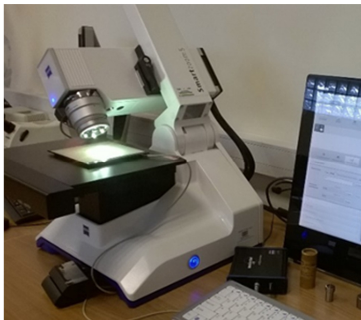
Figure 5. Measuring microscope used for observing wear degree of cutting insert.
