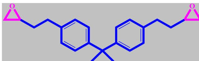
**Figure 3.** Chemical structure of diglycidyl ether bisphenol-A (DGEBA) epoxy resin.
