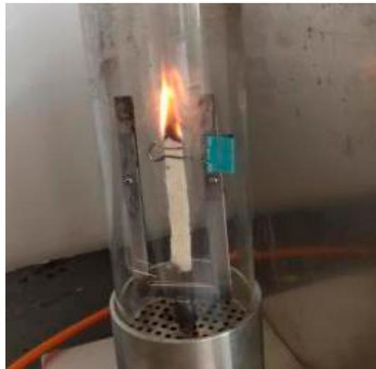
Figure 2. Testing of flame-retardant properties of the composites.
