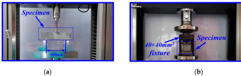
**Figure 2.** Loading setup of the flexural strength (a) and compressive strength tests (b).
