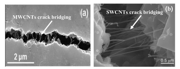
**Figure 11.** Crack bridging by CNTs in  $Si_3N_4$  + CNT systems, [50,68]. Reproduced from Refs. 50 and 68 with permission from John Wiley and Sons and Elsevier, respectively. (**a**) crack bridging by MWCNTs [68]; (**b**) crack bridging by SWCNTs [50].
