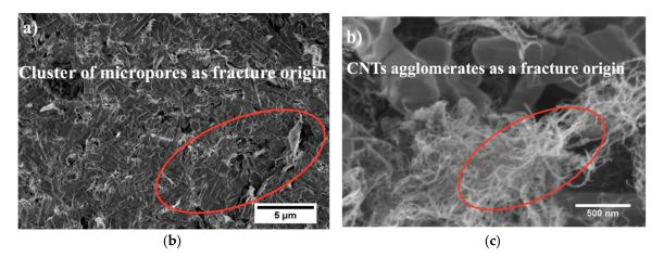
**Figure 8.** Fracture origins of 3 wt.% MWCNT-reinforced Si<sub>3</sub>N<sub>4</sub>: (**a**) area with micropores (**b**) large agglomerate of MWCNTs. (Authors'work)
