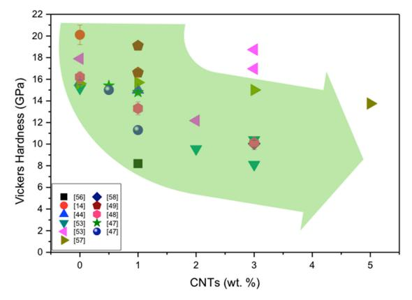
**Figure 6.** Vickers micro-hardness of CNT-reinforced silicon nitride composites according to the results of different investigations. The green highlighted arrow indicates the decreasing tendency of Vickers hardness of  $Si_3N_4$  composites with increasing CNTs content. The details concerning the processing route of the preparation of investigated composites are illustrated in Table 2.
