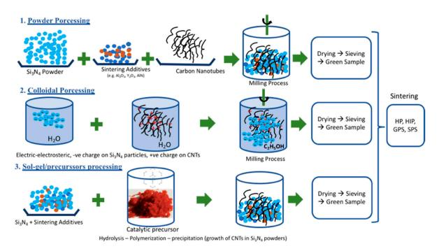
Figure 3. Illustration of the main processing routes used for the processing of  $Si_3N_4$  + CNT composites.
