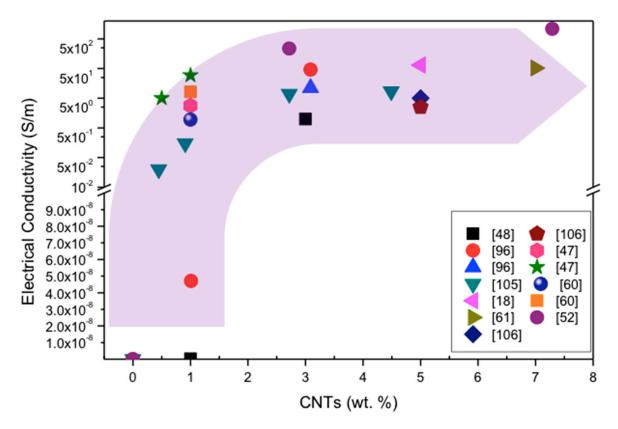
**Figure 15.** Electrical conductivity of CNT-reinforced silicon nitride composites. The processing routes for the preparation of investigated materials are illustrated in Table 5. The purple highlighted arrow indicates the increasing tendency of electrical conductivity of  $Si_3N_4$  composites with increasing CNTs content in the matrix.
