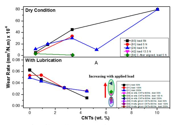
**Figure 12.** Influence of the CNTs addition on the wear rate of  $Si_3N_4$  + CNT composites reported by different researchers.
