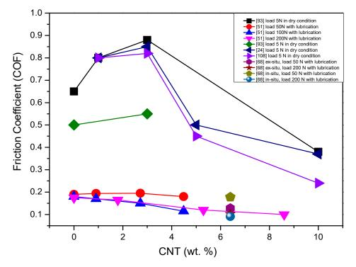
**Figure 13.** Influence of the CNTs addition on the coefficient of friction during the tribological test of  $Si_3N_4 + CNT$  composites reported by different researchers.
