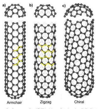
**Figure 2.** Three types of carbon nanotubes (CNTs): (a) armchair (n, m) = (5, 5); (b) zigzag (n, m) = (9, 0); (c) chiral (n, m) = (10, 5) [32]. Reproduced from Ref. [32] with permission from Taylor and Francis.
