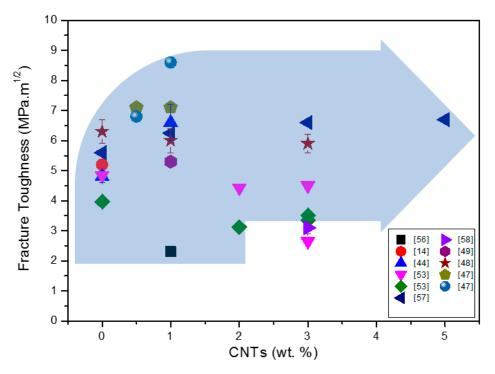
Figure 9. Fracture toughness of CNT-reinforced  $Si_3N_4$  composite measured by indentation fracture techniques. The blue highlighted arrow indicates the increasing tendency of fracture toughness of  $Si_3N_4$  composites with increasing CNTs content. The processing routes for the preparation of investigated materials are illustrated in Table 4.
