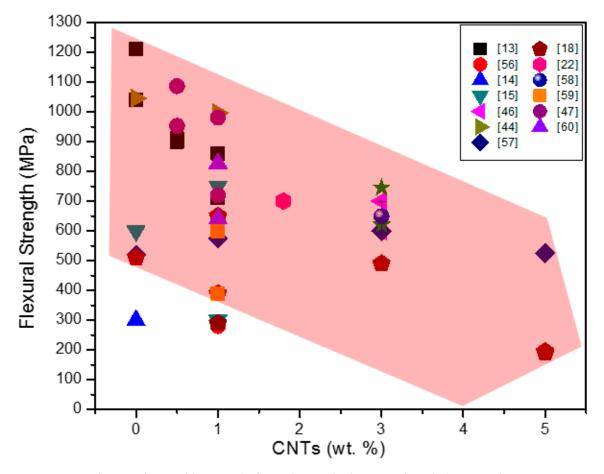
**Figure 7.** Influence of CNT addition on the flexural strength of CNT-reinforced silicon nitride composites. The results are based on 3-point bending test except the source [44] which is based on 4-point bending strength. The highlighted arrow indicates the decreasing tendency of flexural strength of  $Si_3N_4$  composites with increasing CNT content. The processing route for the preparation of investigated materials is illustrated in Table 3.
