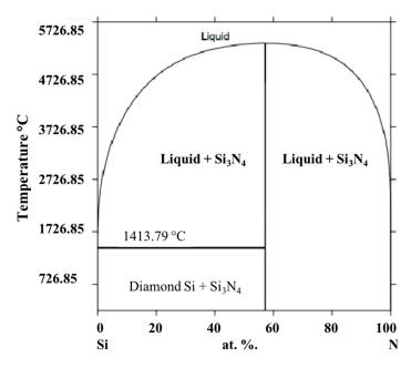
Figure 1. Calculated phase diagram of Si-N system based on [25].
