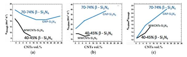
**Figure 14.** Thermal conductivity of CNT- and graphene nanoplatelets (GNP)-reinforced  $Si_3N_4$ : (a) through-thickness; (b) in-plane; and  $K_{in-plane}/K_{through-thickness}$  ratio, (c) silion nitride composites with MWCNTs and GNP as a function of carbon nanostructures, based on [94].
