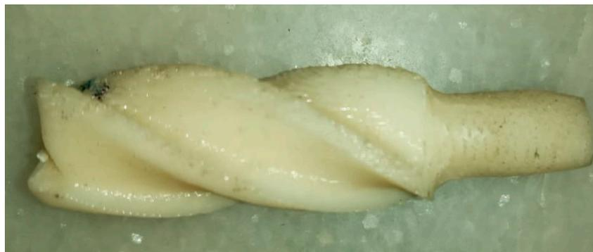
**Figure 1.** As-printed acrylonitrile-butadiene-styrene (ABS) end-mill tool.
