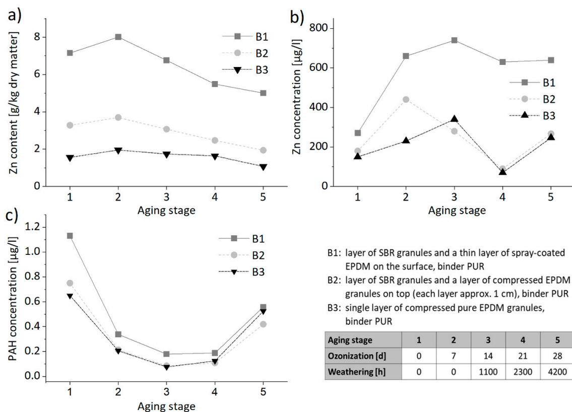
**Figure 4.** Trend of (a) Zn content in solid matter in the course of the artificial weathering of three types of sports floorings (B1 to B3), as well as release of (b) Zn and (c) PAH measured in the eluates of intermittent batch leaching tests at L/S (liquid-to-solid ratio) of 2 L/kg during artificial weathering.
