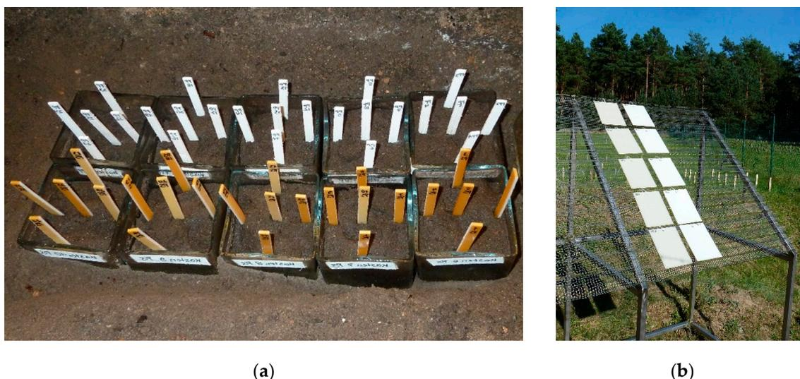
**Figure 7.** Application of different weathering scenarios: (a) soil bed test with flame-protected PP and PS samples and (b) real weathering experiments to evaluate the release of polybrominated flame retardants.
