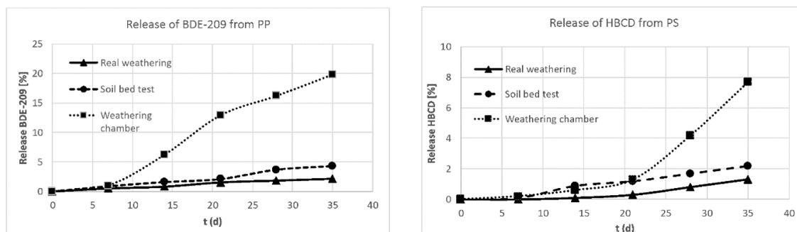
**Figure 6.** Release of selected polybrominated flame retardants from PP (left) and PS (right) samples under different environmentally relevant conditions.
