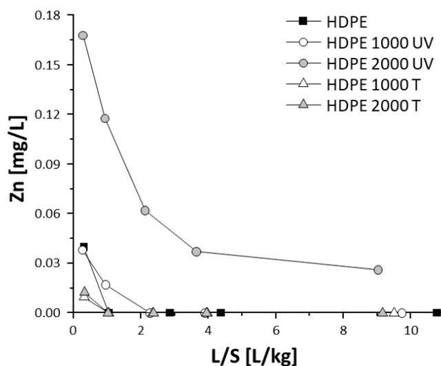
**Figure 5.** Release of Zn as a function of the liquid-to-solid ratio from high-density polyethylene (HDPE) granules in a column leaching experiment. The greatest release was observed in HDPE particles after 2000 h combined thermal and UV irradiation exposure. Converted to cumulative release, the displayed concentrations correspond to approx. 1% of the total Zn content [88].
