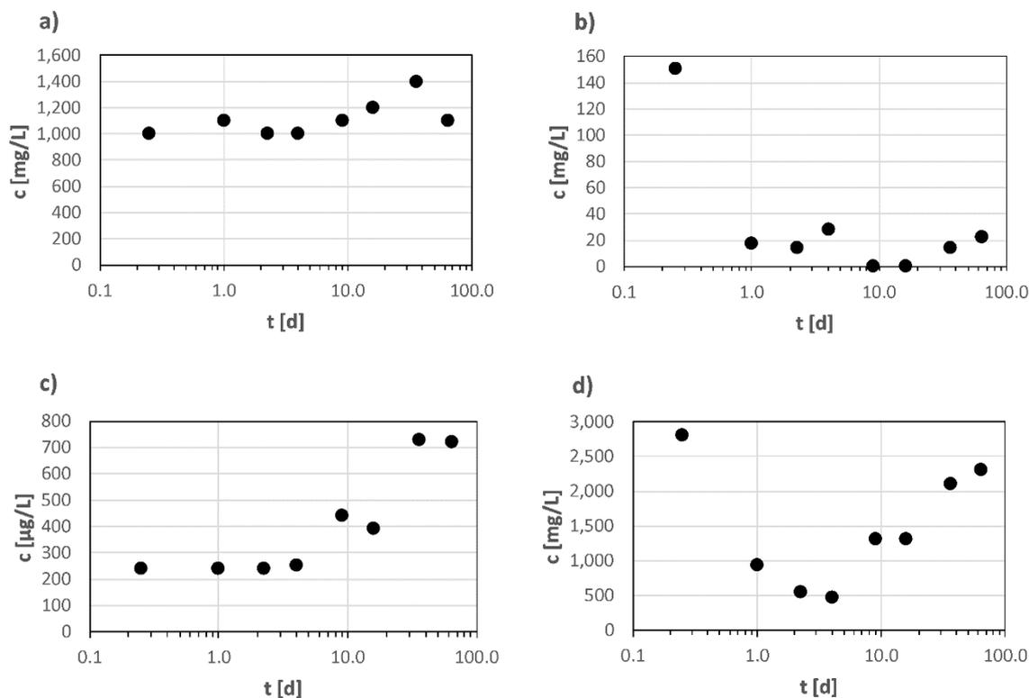
**Figure 2.** Examples of concentration patterns in elute fractions from the dynamic surface leaching test that indicate different release mechanisms as described in [40]. On the  $x$ -axis, the period of water exchange in days is shown for (a) a process controlled by water solubility, (b) first flush (c) a diffusion-controlled process, and (d) first flush combined with a diffusion-controlled process.
