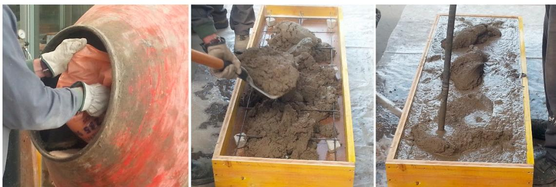
**Figure 6.** Manufacture mortar (left), placing of the mortar (center) and mortar compaction (right).
