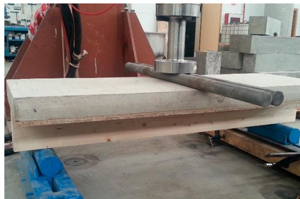
**Figure 9.** Flexural failure test set up.
