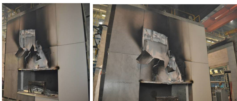
Figure 5. Ventilated facade model view after the fire source was extinguished and the test was completed.
