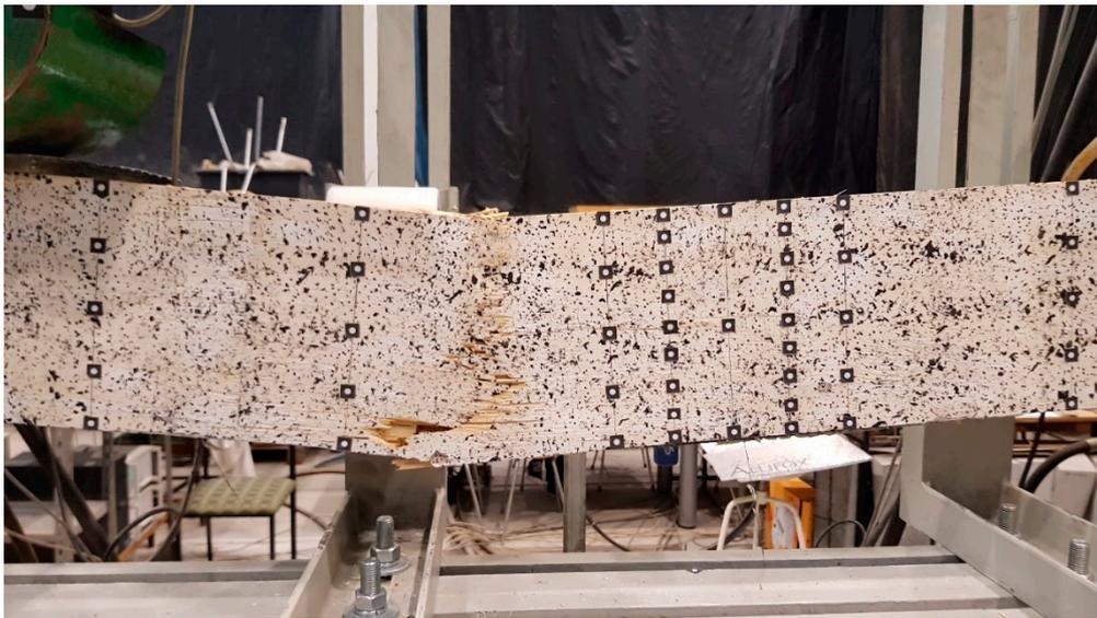
**Figure 7.** An example of a reinforced beam failure (tension + compression).
