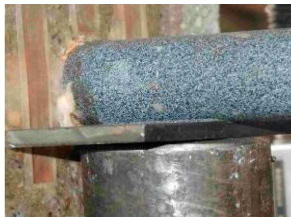
**Figure 4.** Extrusion of polyethylene (PE) plastic dowel coating during loading test of beam with inserted dowel.
