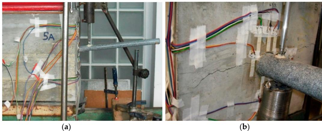
Figure 11. Damage of testing beam: (a) No.1—dowel  $\varnothing$  20 mm; (b) No.4—dowel  $\varnothing$  40 mm.
