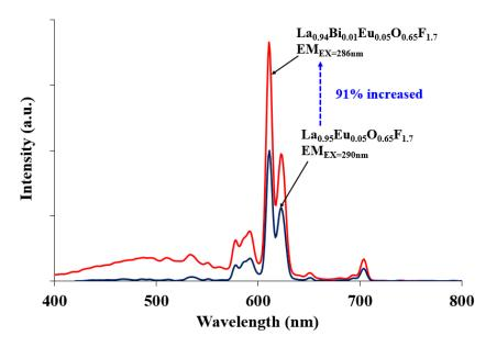
$\textbf{Figure S1.} \ \ \text{The integrated emission intensities of $La_{0.95}Eu_{0.05}O_{0.65}F_{1.7}$ and $La_{0.94}Bi_{0.05}O_{0.65}F_{1.7}$ phosphors.}$
