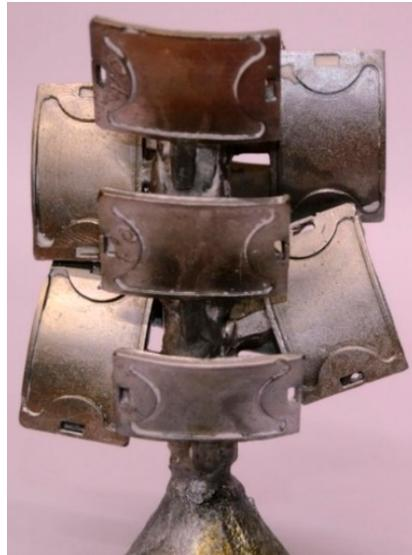
**Figure 14.** An example of the application of PE-wax modified by bentonite for the production of an aluminum alloy casting in the lost-wax casting process.
