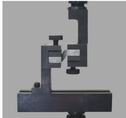
Figure 5. Fixture of shear test device.
