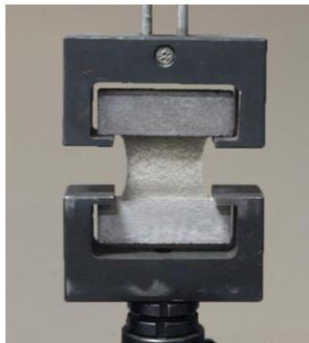
**Figure 4.** Fixture of tensile at elongation test device.
