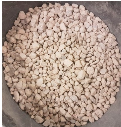
Figure 1. Recycled coarse aggregate obtained after thermal and mechanical treatment.
