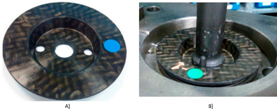
**Figure 16.** (A) Redesign of the CFRTP part. (B) CFRTP Part (PA 6 and P69) ready to begin the test.
