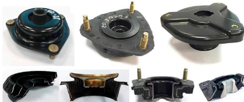
Figure 4. Automotive anti-vibration products: vulcanized rubber and steel.
