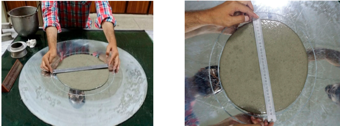
Figure 9. Flow test of self-compacting cementitious mortar.
