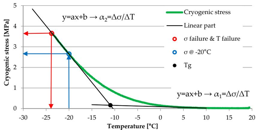
Figure 6. Graphical explanation of data assessment from TSRST.
