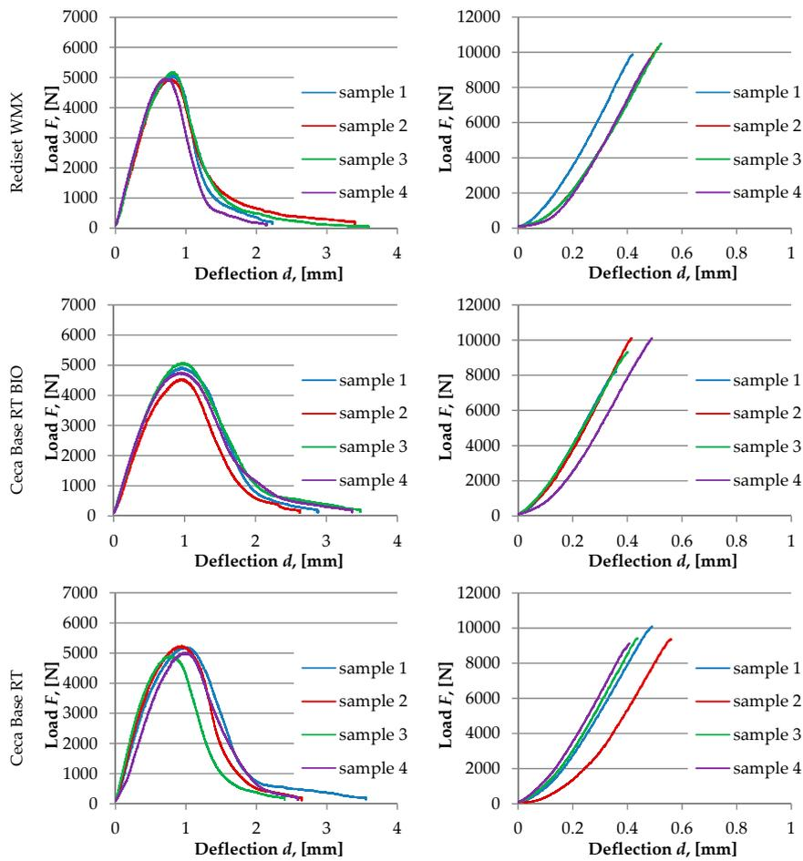
**Figure 10.** Selected results from the SCB test. Load/deflection curves for samples with a 10-mm notch. Left column: test temperature +10 °C. Right column: test temperature −20 °C.
