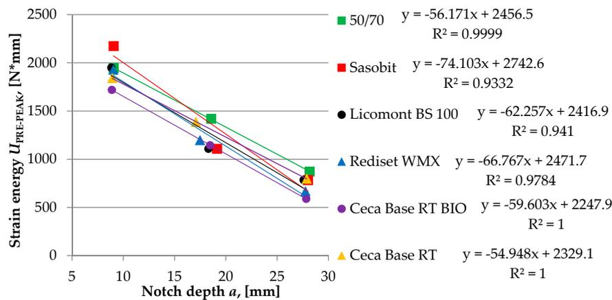
Figure 12. The graphical explanation of J<sub>C</sub> calculation from the SCB test at −20 °C.
