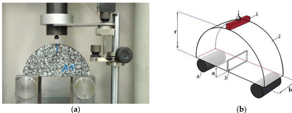
**Figure 7.** Semi-circular bending test (SCB) with the displacement strain rate setup: (a) photograph of the test setup. (b) Layout of the supports and loading point (1—loading rod, 2—sample, 3—notch, and 4—supporting rods).
