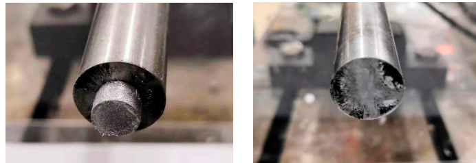
Figure 5. Comparison of specimens before and after SHPB experiment.
