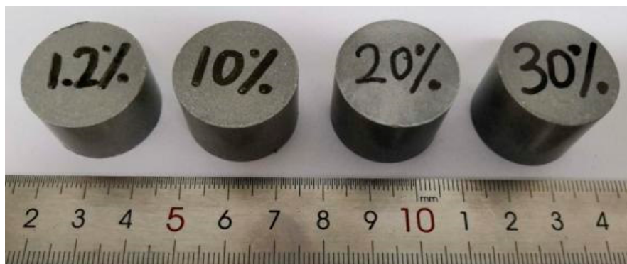
Figure 1. Specimens of PTFE/Al with different porosity.
