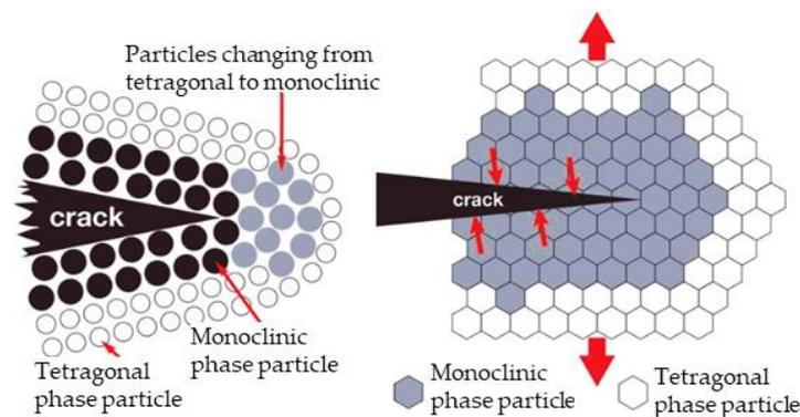
Figure 12. Transformation toughening mechanism in zirconia [29].
