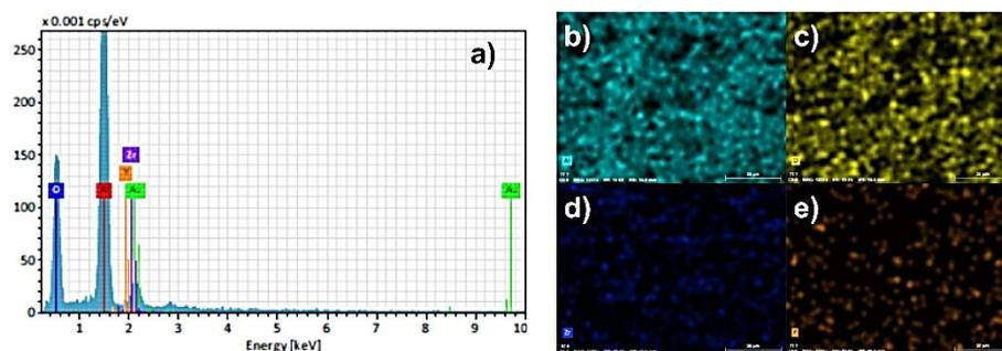
**Figure 9.** (a) EDS spectra of surface fracture of  $Al_2O_3$ - $ZrO_2$  ceramics with 1 wt. % of  $ZrO_2$  and corresponding element mappings: (b) Aluminum (Al); (c) Oxygen (O); (d) Zirconium (Zr); (e) Yttrium (Y).
