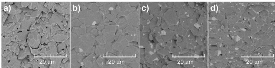
**Figure 7.** Surface fracture of  $Al_2O_3$ - $ZrO_2$  composite ceramics with different content of  $ZrO_2$ : (a) 0 wt. %; (b) 1 wt. %; (c) 5 wt. %; (d) 10 wt. % prepared by slip casting and sintering at 1650 °C.
