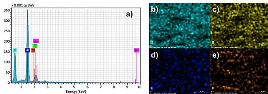
**Figure 10.** (a) EDS spectra of surface fracture of  $\text{Al}_2\text{O}_3\text{-ZrO}_2$  ceramics with 5 wt. % of  $\text{ZrO}_2$  and corresponding element mappings: (b) Aluminum (Al); (c) Oxygen (O); (d) Zirconium (Zr); (e) Yttrium (Y).
