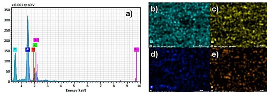
**Figure 11.** (a) EDS spectra of surface fracture of  $\text{Al}_2\text{O}_3\text{-ZrO}_2$  ceramics with 10 wt. % of  $\text{ZrO}_2$  and corresponding element mappings: (b) Aluminum (Al); (c) Oxygen (O); (d) Zirconium (Zr); (e) Yttrium (Y).
