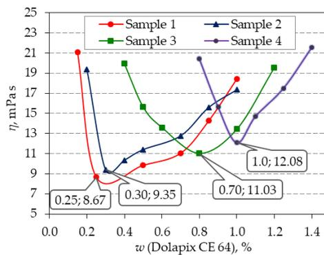
**Figure 6.** Influence of amounts of Dolapix CE 64 dispersant (wt. %) on apparent viscosity ( $\eta$ ) of the 70 wt. % suspensions with ceramic powder composition of sample 1: 100 wt. %  $\text{Al}_2\text{O}_3$ ; sample 2: 99 wt. %  $\text{Al}_2\text{O}_3$  + 1 wt. %  $\text{ZrO}_2$ ; sample 3: 95 wt. %  $\text{Al}_2\text{O}_3$  + 5 wt. %  $\text{ZrO}_2$ ; sample 4: 90 wt. %  $\text{Al}_2\text{O}_3$  + 10 wt. %  $\text{ZrO}_2$ .
