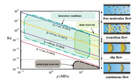
**Figure 9.** Rarefied gas flow type under different conditions. This can be divided into free molecular flow ( $K_n > 10$ ), transition flow ( $0.1 < K_n < 10$ ), slip flow ( $10^{-3} < K_n < 0.1$ ), and continuous flow ( $K_n < 10^{-3}$ ).
