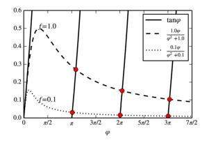
**Figure 1.** Graphical representation of the characteristic Equation (11). The solid lines represent the tangent function of  $\phi$  and the dotted lines represent the fraction with different values of the non-dimensional number *f*. The red circles represent the characteristic roots of Equation (11). As *f* decreases, each characteristic root tends to be a positive integer multiple of  $\pi$ .
