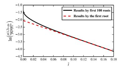
**Figure 2.** The truncation result of the analytic solution. The solid line represents the result of the truncation for the first 100 characteristic roots of Equation (11) and the dotted line represents the result of the truncation for the first characteristic root. When the dimensionless time is greater than 0.1, there is little difference between the two curves.
