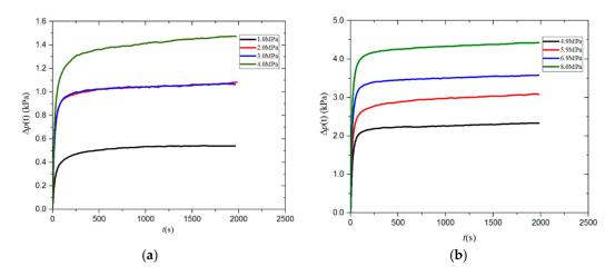
**Figure A1.** Pressure difference signal ( $\Delta p(t)$ ) for shale particle sample 1 measured by the differential pressure transducer under pressures of 1–8 MPa. (**a**) average pore pressure under 1–4 MPa with smaller  $\Delta p_{fi}$  (**b**) average pore pressure under 5–8 MPa with larger  $\Delta p_{fi}$ .
