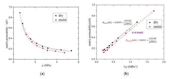
**Figure 11.** Matrix permeability of dry and moist (1.5% water) samples of shale sample 1 under different pressures. (a) Matrix permeability vs. pressure. The dotted lines are the results of fitting using the Klinkenberg equation. (b) Matrix permeability vs. 1/*p*.
