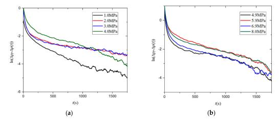
**Figure A2.** Logarithmic pressure decay curve,  $ln(\Delta p_f - \Delta p(t))$ , for shale particle sample 1 under pressures of 1–8 MPa. (a) average pore pressure under 1–4 MPa; (b) average pore pressure under 5–8 MPa.
