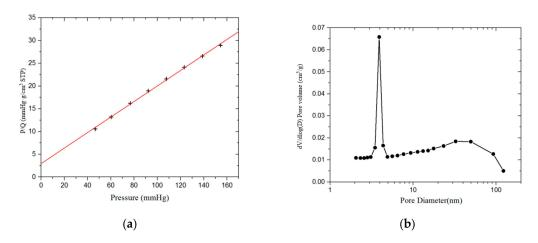
**Figure A3.** Nitrogen adsorption of sample 1 measured by an ASAP 2420 instrument (Micromeritics Instrument Corp., Norcross, GA, USA). (a) Langmuir surface area plot; (b) BJH desorption dV/dlog(D) pore volume.
