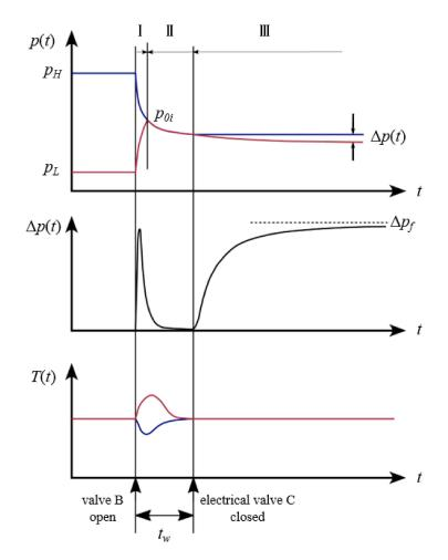
**Figure 4.** Graphs of the pressure p(t) of the reference chamber and sample chamber, the pressure difference signal  $\Delta p(t)$  measured by the differential pressure transducer, and the gas temperature T(t) in the pipe.
