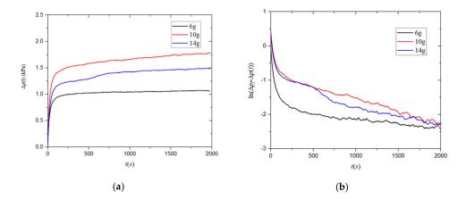
**Figure 6.** (a) The pressure difference signal  $\Delta p(t)$  and (b) logarithmic pressure decay curve for sample 1 measured at a pressure of 3 MPa and a temperature of 30 °C The black, red, and blue lines indicate sample masses of 6, 10, and 14 g, respectively.
