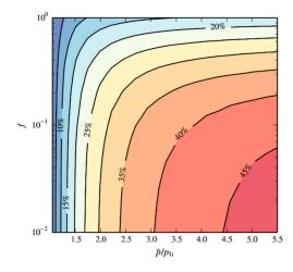
**Figure 12.** The relative error in the calculated permeability due to ignoring gas compressibility. For systems with a smaller dimensionless number *f*, when the system initial pressure ratio is large, ignoring the gas compressibility leads to a larger error in the calculated permeability.
