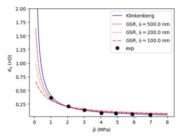
**Figure 13.** A comparison of the permeability fitting using the general slip regime (GSR) model and the Klinkenberg model. The characteristic flow scales  $l_f$  used for the fitting with the GSR model were 100, 200, and 500 nm.
