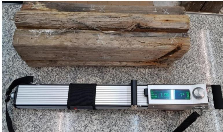
Figure 3. IML RESI PD-400S device used in tests.
