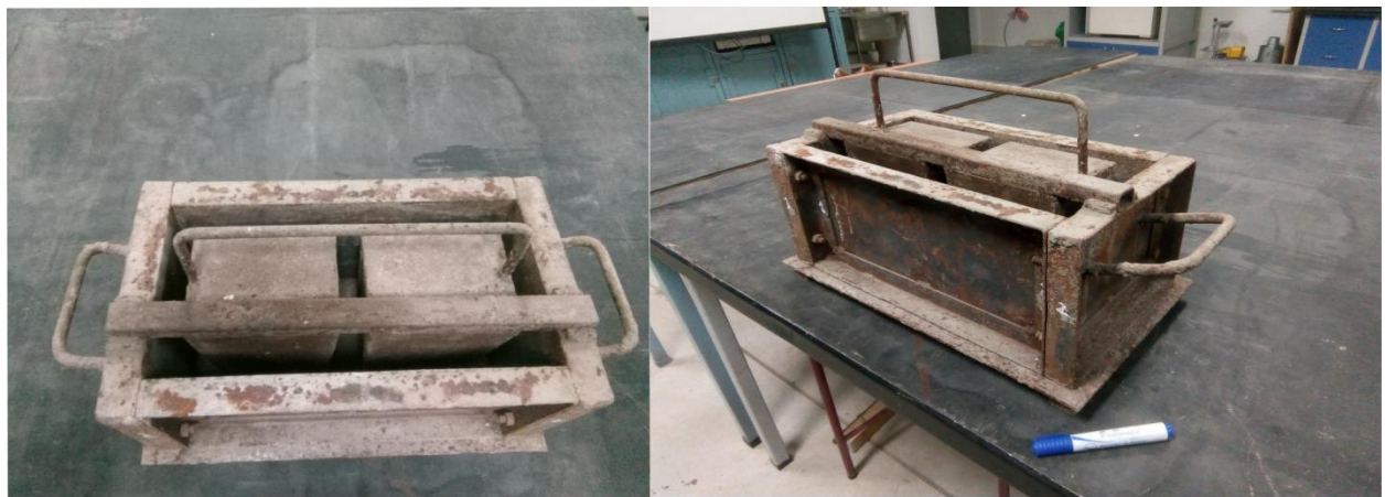
Figure S1. Formwork used in the construction of the blocks.
