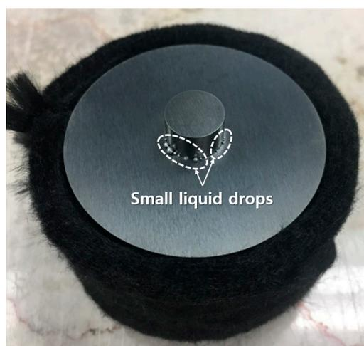
**Figure 4.** Photograph of cemented mold of semisolid sintered Al-SUS316L composite.
