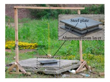
Figure 3. Sketch of the experimental setup.
