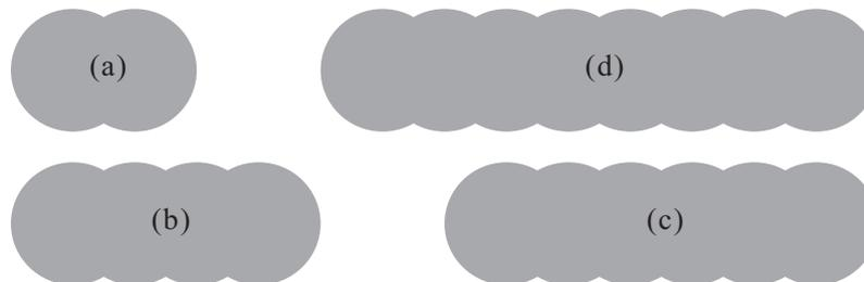
**Figure 14.** Clump templates used to create concrete aggregates with shape factors equal to: (a) 1.5; (b) 2.5; (c) 3.5; and (d) 4.5.
